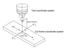
There are two ways to find the surface. Using the first method, the tip of cutting head doesn't touch the surface; the system reads the distance from the analog input signal of the sensor. Using the second method, the tip of cutting head touches
