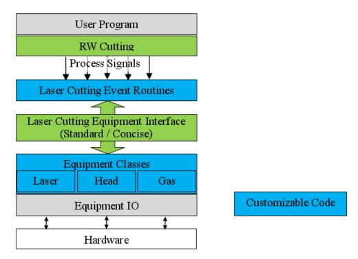
There are two sets of laser equipment interfaces: concise and standard interfaces. Standard laser equipment interfaces define all the common functions for mainstream laser equipment, and they are available for the laser cutting system with standard equipment task. Concise interfaces are a subset of the standard interfaces, which includes basic functions. They are provided as default equipment interfaces for laser cutting systems without standard equipment task.
