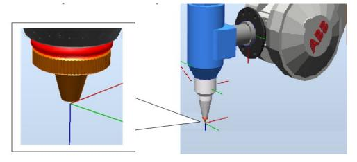
There are 2 ways to define TCP: manually and automatically. Bullseye is recommended to be used to define the TCP automatically.
